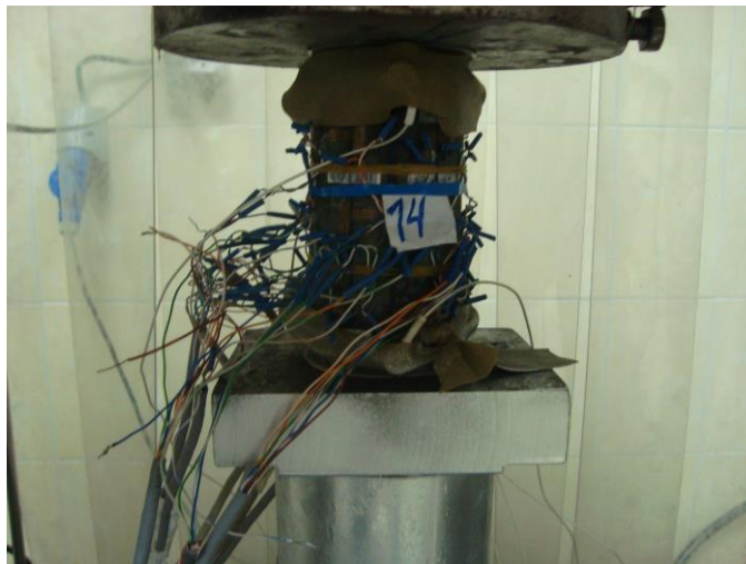
Fig. 12. Rock sample in the loading process
