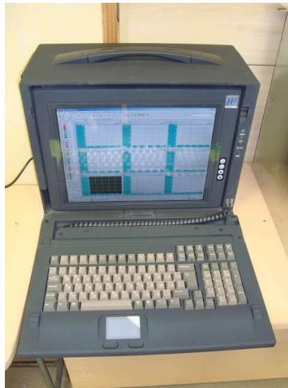
Fig. 10. Acoustic-emissive measurement complex A-Line 32D
