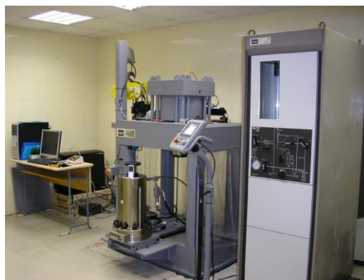
Fig. 2. MTS-816 load system in Laboratory on Geodynamics FEFU
