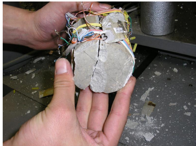
Fig. 4. Macrofailure character of dacite sample (N 3)
