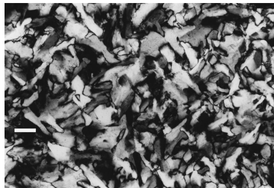
Fig. 1. Coesite starting material, crystallized from silica glass cylinder at 1000°C, 3.6 GPa, for 24 h. Scale bar = 100 \mu\text{m} . Crossed polarized light.
