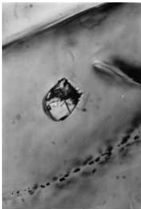
Fig. 1. A group of secondary inclusions and a larger primary melt inclusion in clinopyroxene from Kovdor ijolite. The primary inclusion is \sim 40 \mu\text{m} across.
