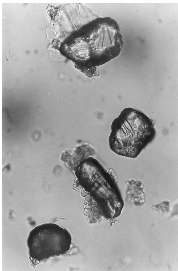
Fig. 2 Run products from an outer capsule: diamond powder (grain size 40–60 microns) and carbonate particles attached to the surface of diamond grains
