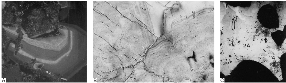
Fig. 10. Photomicrographs illustrating various types of distribution of compositional areas in carbonate minerals. (A) Cathodoluminescence photomicrograph illustrating concentric growth zoning in calcite (width is 300 \mu\text{m} ); (B) Transmitted light photomicrograph of calcite stained with alizarin red S and Potassium ferricyanide, illustrating alternating concentric growth zones in outer parts of crystals and recrystallized patches in crystal interiors (see interior of crystal on left. Width is 0.88 mm); (C) Back scattered electron image of baroque dolomite/ankerite with radiating areas of recrystallization and fluid inclusion entrapment. Dark irregular core (filled arrow) is corroded and partially replaced by late bright phase (4) in radiating pattern. Intermediate brightness ankerite (2A) dominates. Numbers are as those in Wojcik et al. (1997). Width is 260 \mu\text{m} . Modified from Wojcik et al. (1997).
