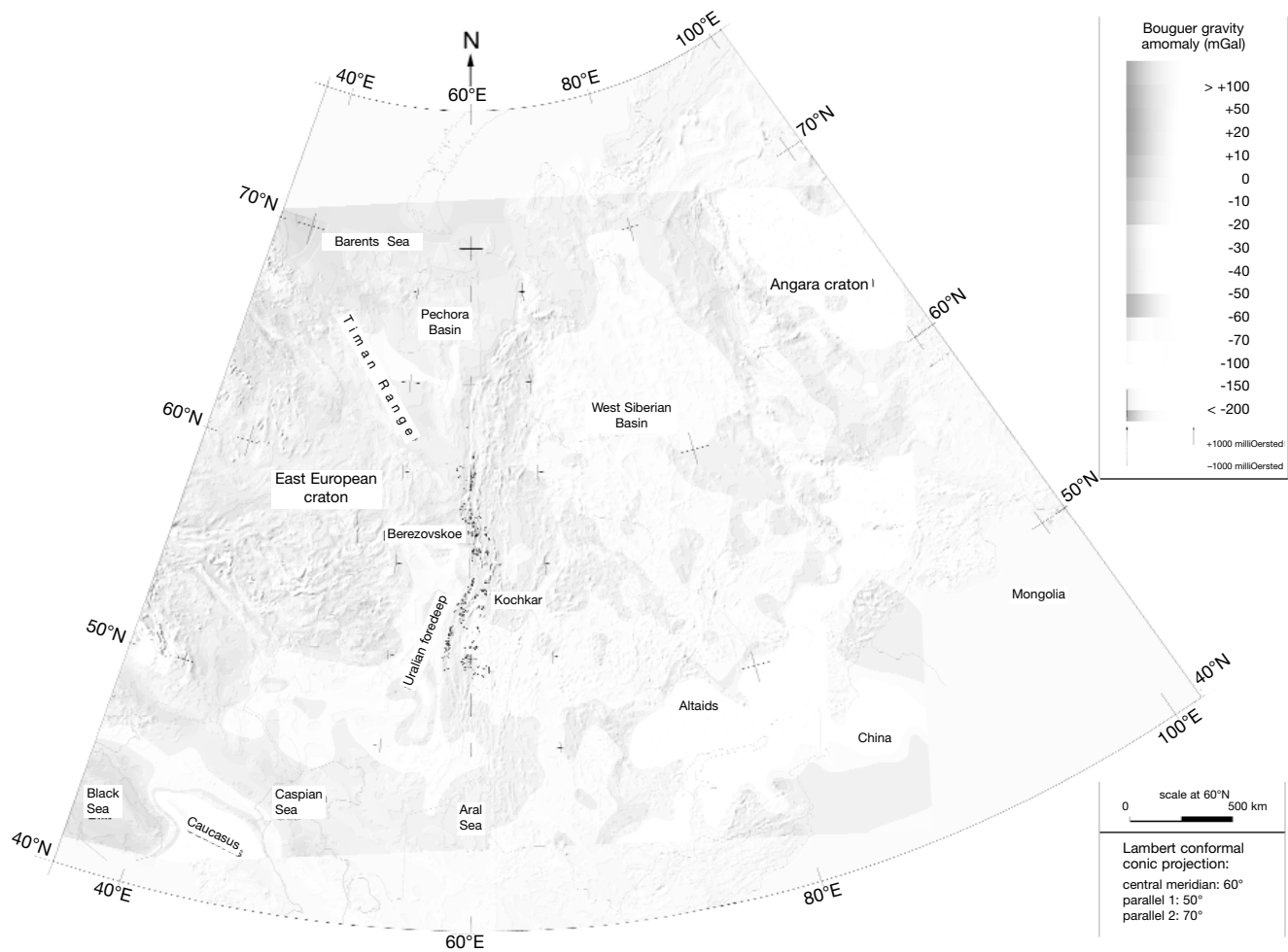
FIG. 12. The Bouguer gravity anomaly pattern of the region between the East European and Angara cratons (Ministry of Geology, USSR, 1977a) superimposed on the magnetic anomaly pattern in shaded relief (Fig. 9). A broad Bouguer gravity anomaly high, from the Barents Sea to the southeast, transects the Urals. It separates the southern Urals from the middle Urals at about 55° N. Gold deposits are shown as dots.
