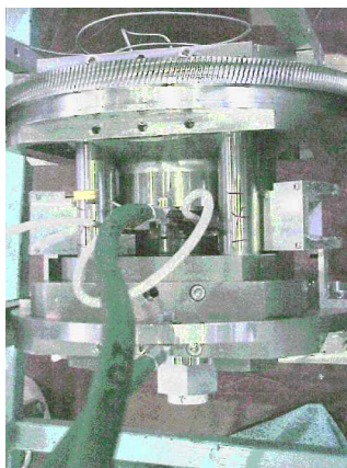
FIG. 1. (Upper) Schematic design of the anvil assembly of the Paris-Edinburgh cell. (Middle) Schematic design of internal heating components. (Lower) Photographs of the Paris-Edinburgh cell with power supplies connected.
