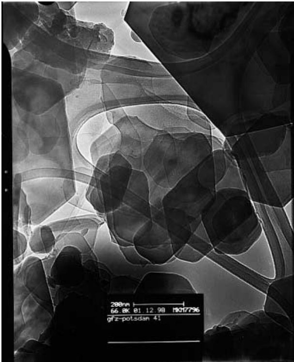
Fig. 2 TEM bright field image of run product 98-41 showing chlorite and chloritoid, both with hexagonal crystal shape
