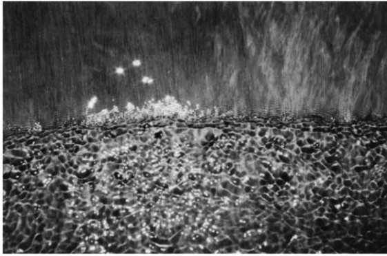
Fig. 3. Photograph looking vertically down on the hydraulic jump at the commencement of the region of hydraulic adjustment. The disturbed nature of flow is evident in at least the surface of the hydraulic jump. Flow is in the direction from uniform laminar flow to the disturbed flow.
