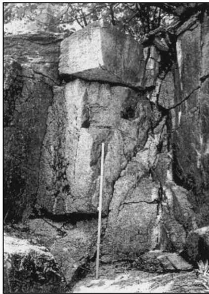
Fig. 7. Changes in joint appearance. (A) Sharp-edged, straight joints in fresh granite (note person for scale). (B) Stained, sharp-edged, and straight joint in slightly weathered granite. (C) Rounded exposure and joint edges in fresh granite. (D) Weathering- and stress-induced joints in moderately weathered granite. (E) Rounded-edged, open joints in highly weathered granodiorite. (F) Iron stained joint locations in completely weathered granite. Scales used: metre stick, 1 m; Nolan hammer, 45.7 cm.
