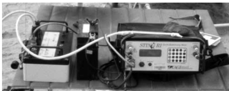
Fig. 2. Photograph showing a close-up of the Sting/Swift resistivity system. The Sting (on the right) is the resistivity meter and data logger. The Swift (on the left) is the switching system that connects to the multiple electrode cables and allows the Sting to select which four of the 56 or more electrodes to use for each resistivity measurement. In the centre is the 12 V motorcycle battery that provides electricity for the measurements.
