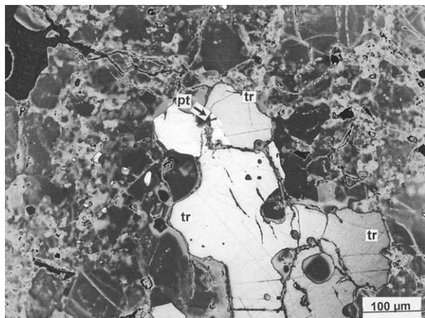
Fig. 5. Polycrystalline troilite grain with included pentlandite. The bulk of the troilite (tr) is a single crystal (light gray), a second crystal of troilite forms a darker-shaded patch at the center of the image (medium gray). Pentlandite (pt, white) occurs immediately to the left of the second troilite crystal. Mafic silicate grains (medium to dark gray) surround the sulfide assemblage. Reflected light.
