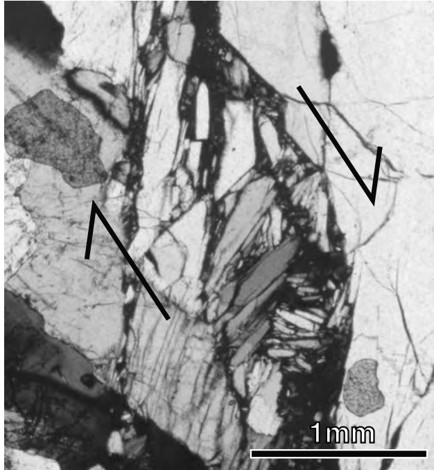
Figure 16. Thin section optical photomicrograph (cross-polarized light) showing the process of erosion of the transition zone during the shearing. Particles are released from the transition zone and incorporated in the gouge material. \sigma_1 and \sigma_3 are parallel to vertical and horizontal directions, respectively. \sigma_3 = 40 MPa, \epsilon_1 = 0.045 .
