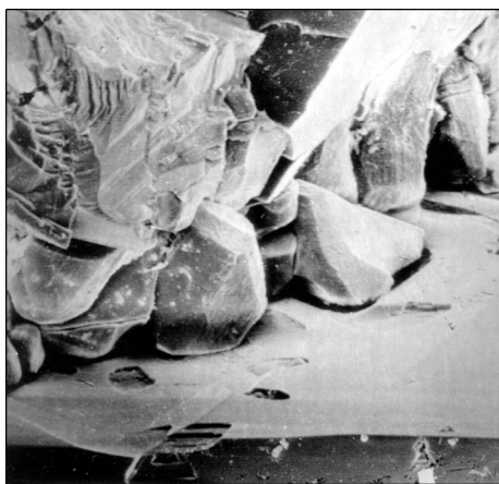
Fig. 8. Forsterite crystals on diamond surface (system K_2CO_3 - Mg_2SiO_4 -C, run no. 15), \times 440 .
