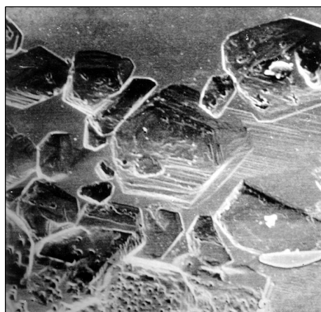
Fig. 9. Induction surfaces of diamond and forsterite cogrowth on {111} face of seed crystal ( K_2CO_3 - Mg_2SiO_4 -C system, run no. 14), \times 220 .
