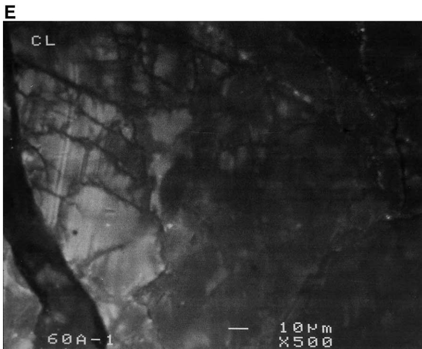
Fig. 4. Optical microscopic (A), SE (B), BSE (C), and CL (D) images of the 60 GPa sample. Relatively widely spaced (10–20 \mu\text{m} ), grain-pervasive fractures are characteristic of this sample. The CL intensity is also rather low in the magnified CL image (E). The scale of (A) is the same as (B).
