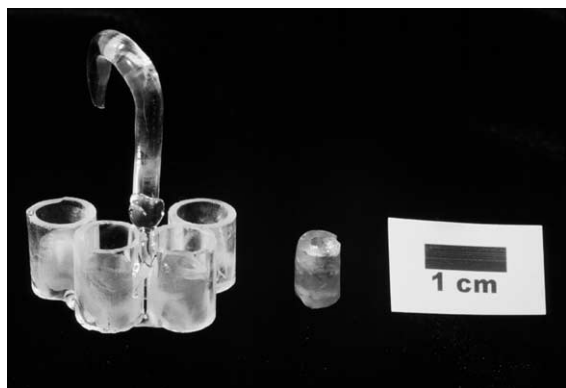
Fig. 2. Photo of sample assembly loaded with three San Carlos olivine crucibles. A single crucible is shown to the right of the assembly; 1 cm scale bar for reference.
