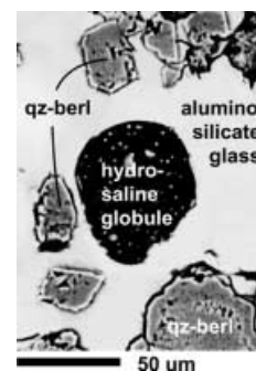
Fig. 5. Backscatter electron image of a globule of immiscible B- and F-rich liquid and aluminosilicate glass quenched at 550 °C and 0.2 GPa
