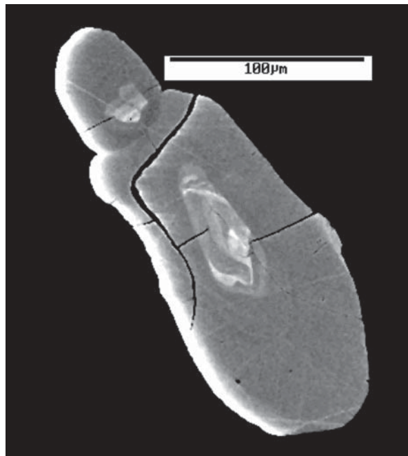
FIGURE 11. Natural zircon crystal with composite Grenville age cores and Ordovician age rims. From Winding Stair Gap granulite grade metapelite, southern Appalachian Blue Ridge (Miller et al. 1998).
