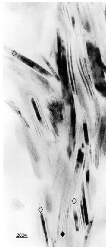
FIGURE 11. HRTEM image of the <0.1 \mu\text{m} size-fraction from McGerrigle Mountains Pluton anchizone (TM 39) after treatment with n_c = 18 showing R3-ordered structure consisting of thin packets of 3 to 6 non-expandable layers (open diamond with expandable interface with an average spacing of 21–22 Å (white arrows). The black arrows denote the termination of non-expandable packets and conversion to a fully expanded coherent domain.
