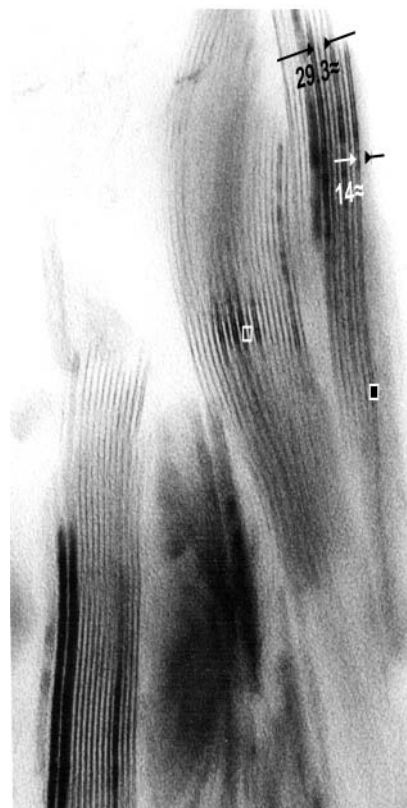
FIGURE 10. HRTEM images of the <0.1 μm size fraction from the McGerrigle Mountains Pluton anchizone (sample TM39) after treatment with n_c = 18 showing a sequence of a corrensite-like, R1-ordered structure consisting of double layers, alternating between non-expandable 14A 2:1 layers (solid squares) and expandable interlayers with average spacing of 29–30 Å (open squares).
