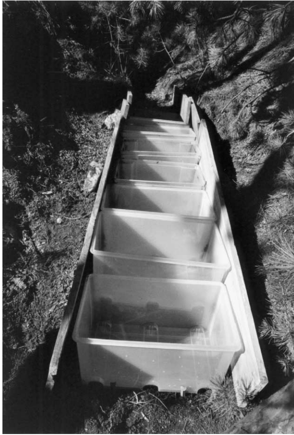
Fig. 4. Sediment trap with a capacity of 500 l.
