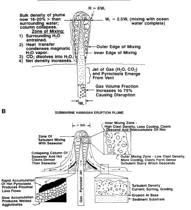
Fig. 4. Submarine hawaiian eruption model developed in this analysis. (A) Formation and emergence of gas/pyroclast jet and development of the zone of mixing. (B) Evolution and collapse of the zone of mixing to form flows, welded agglutinates, and density currents.
