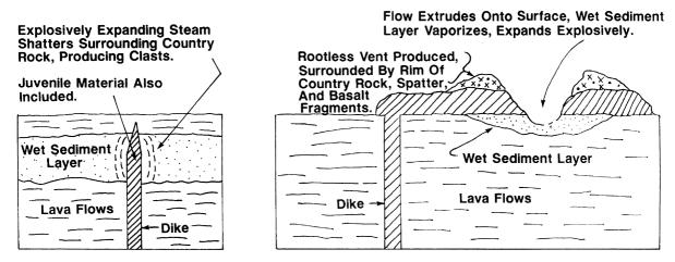
Fig. 9. Processes and environments of bulk interaction steam explosivity.
