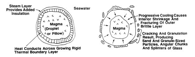
Fig. 8. Processes and environments of cooling-contraction granulation.
