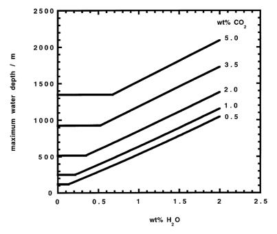
Fig. 3. The maximum depth in the ocean at which an eruption can be of the steady explosive hawaiian-style, shown as a function of the initial magmatic  $H_2O$  content for a series of initial magmatic  $CO_2$  contents. The depth ceases to depend on water content when magma fragmentation takes place solely due the presence of  $CO_2$  bubbles before any  $H_2O$  exsolution has taken place.
