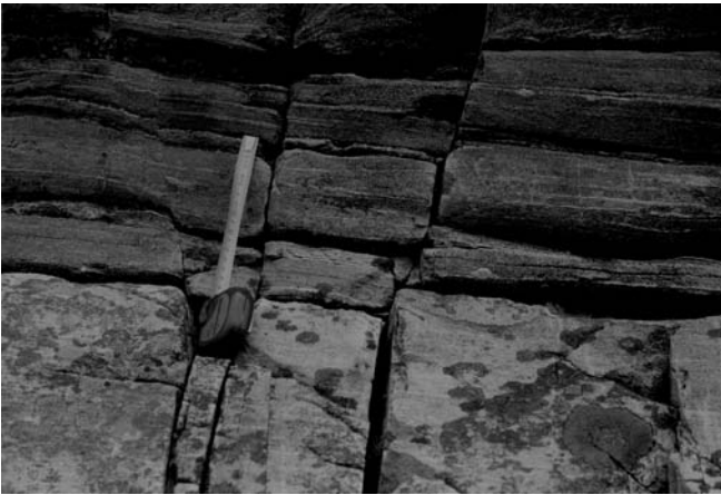
Fig. 6 Development of shear fractures in a vertical section through a mechanically layered host rock, gneiss, on the island of Øygarden, West Norway. Some of the mechanical layers, mainly generated by exfoliation, coincide with the primary layers of alternating dark amphibolite and light quartzo-feldspathic gneiss. The main shear fracture (just to the right of the centre of the photograph) strikes N45°E, and it has an average dip of 72°NW and a vertical displacement of 4 cm. The shear fracture tends to be somewhat steeper in the stiffer (high Young's modulus) layers. View northeast; the length of the steel tape is 0.2 m
