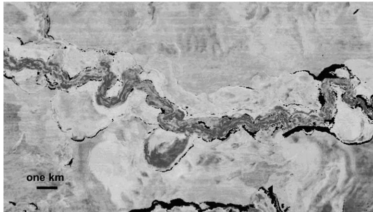
Fig. 3. Time slice of neutral channel, 80 ms below sea floor, offshore Indonesia. Image kindly supplied by Henry Posamentier.
