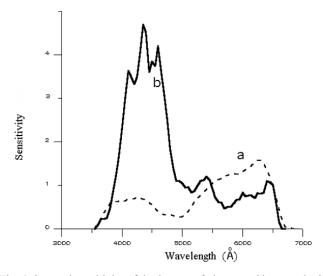
Fig. 4. Spectral sensitivity of the 2 types of plates used here to obtain meteor spectra.
