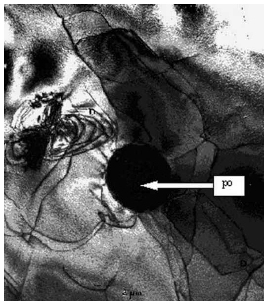
Fig. 3 Relation between pyrrhotite exsolution and sphalerite matrix. Multibeam TEM bright-field image (bd = [111]) with corresponding diffraction pattern (SADP) for the sphalerite matrix and pyrrhotite as well as for dislocations (D). Sample LZf 30/3, Philips CM 200, U = 200 kV
