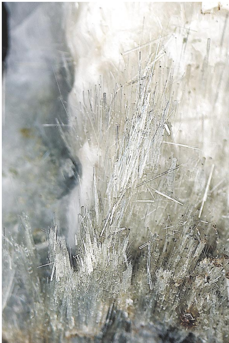
FIG. 2. Acicular crystals of fluorvesuvianite in a calcite matrix. The horizontal dimension of the field of view is 12 mm.
