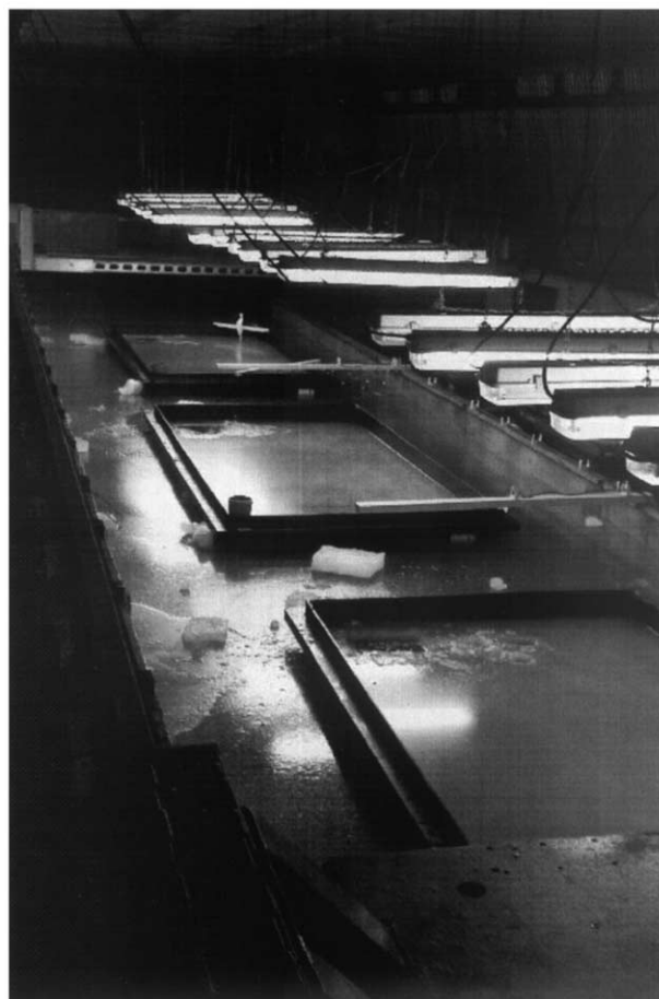
Fig. 1. Experimental setting: three of the four tanks (A, B and C) are shown submerged into a larger basin 2 d after the onset of ice formation (photo: Mats Granskog).
