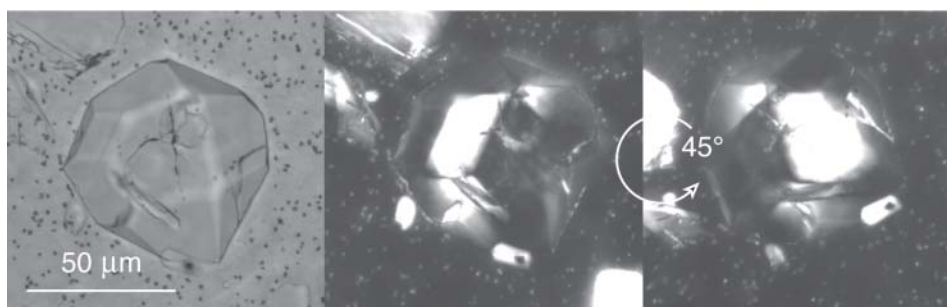
FIGURE 2. Large grossular crystal (70 \mu\text{m} diameter) embedded in epoxy with \{211\} dominating over \{110\} . Run G18 (Milke and Metz 2002), 675 °C, 621 h. Left picture in transmitted light, middle picture with crossed polarizers, right picture with crossed polarizers and turned 45°.
