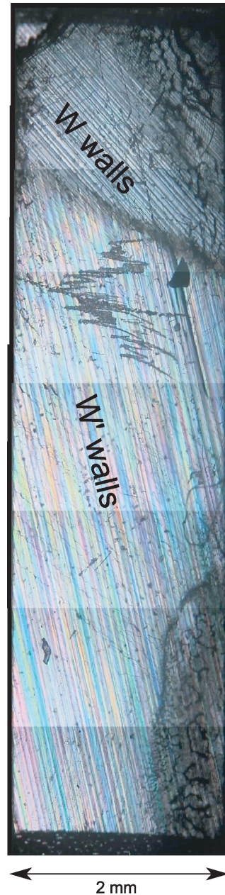
FIG. 1. Optical micrograph of the pure starting material. W walls in the upper portion are perpendicular to the (100)_{\text{mon}} cleavage surface and are characterized by the black-white contrast observed when one set of twins is rotated into extinction. W' walls in the lower portion of the crystal are tilted by an angle of \sim 17^\circ to the surface and are characterized by their birefringent interference colours.
