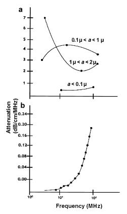
Figure 1. (a) A schematic of acoustic attenuation spectra for three particle-size ranges, a (L). (b) The acoustic attenuation spectrum for water.
