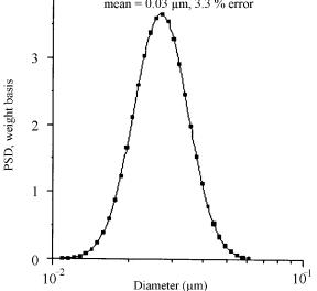
Figure 3. (a) Acoustic attenuation spectrum of a 10 wt.% Silica Ludox standard, at pH 9.3 and 26.7°C. The  $\zeta$  potential measurement was -38 mV. (b) The lognormal particle-size distribution calculated from the attenuation spectrum. The mean size was 0.03  $\mu$ m with a deviation from a lognormal distribution of 3.3%.
