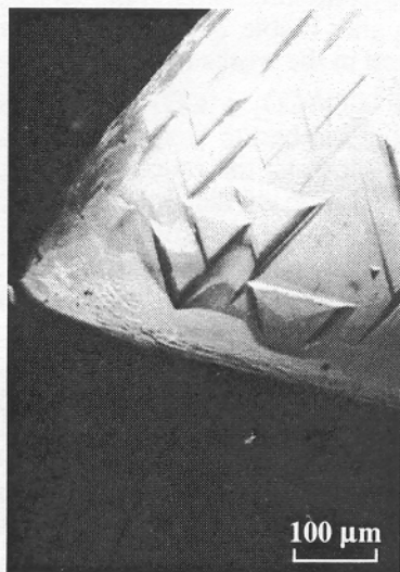
Fig. 1. Negative trigons on the face \{111\} of a diamond crystal etched in the kimberlitic melt.
