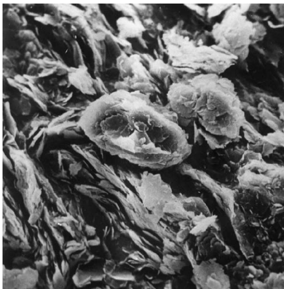
Fig. 9. Spheroidal surface type (rosette structure). Borrowdale, England. Scanning electron microscopy.
