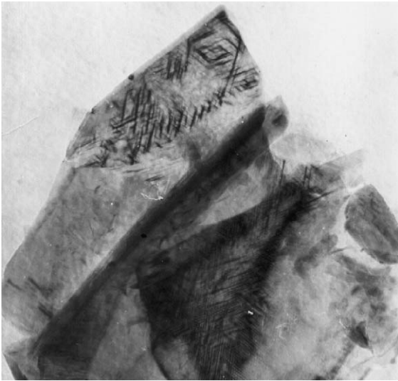
Fig. 6. Rhombic Moire effect resembling growth spirals. Male Vrbno, Czech Republic. Transmission electron microscopy.
