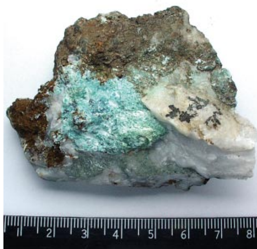
FIG. 2. Pocket of green nickeloan talc in magnesite–quartz vein, Uspenskaya gorka. Scale in cm.
