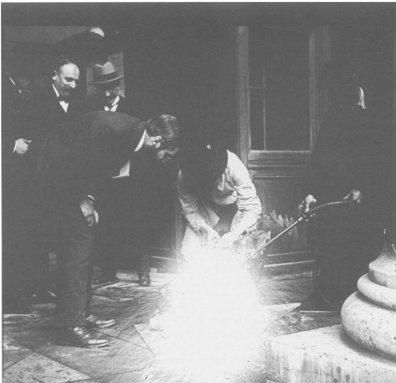
Fig. 20. Cutting the Tamentit meteorite with a soldering torch in the gallery of the MNHN under the watchful eye of Prof. Lacroix (Archives, © Laboratoire de Minéralogie, MNHN).
