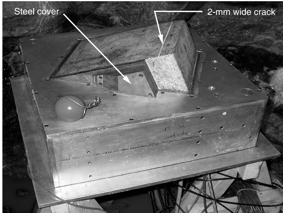
Figure 3. Panel on table at the bottom of the vertical shaft. Sphere at bottom left corner of panel was the anchor for measuring sliding velocity.
