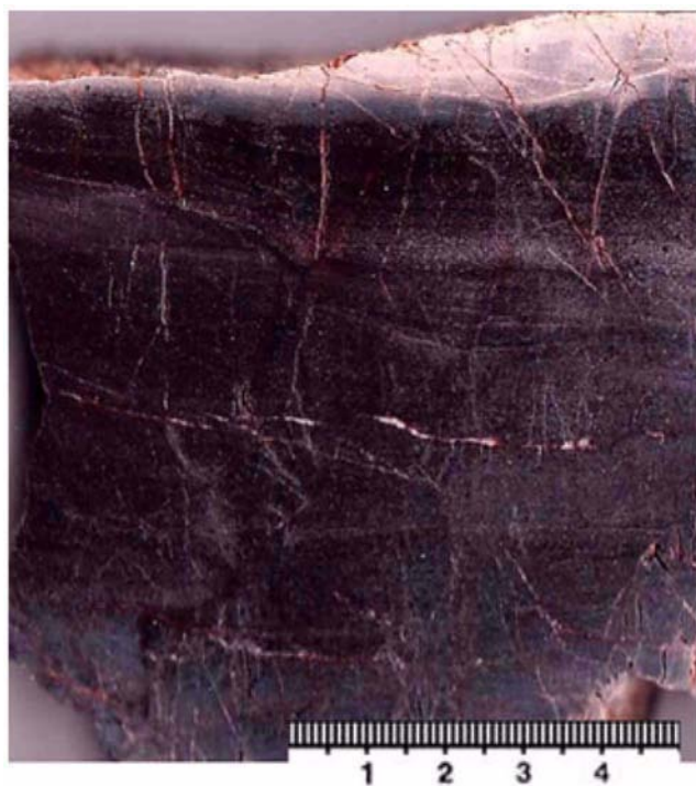
Fig. 5. Cross section of the TM3 bedded-chert, dark-gray to black, well-laminated, containing a large amount of fine vitric tuff materials (whitish bands and dotted grains).
