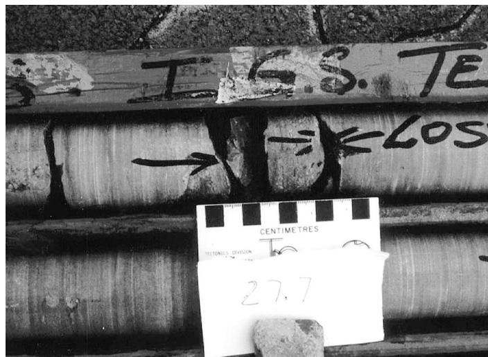
Fig. 7. Photograph of the horizontal fracture on the Campus Test Site as it appears in a core sample.
