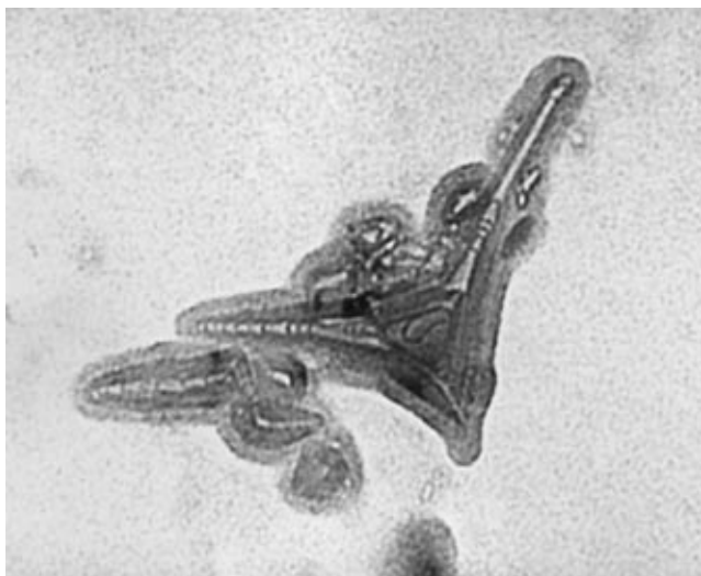
Fig. 4. Combination of a fullerite structure with segmented carbon nanotubes (magn. 300 000).
