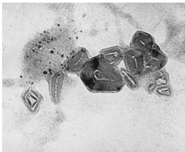
Fig. 2. Fullerite multilayer structures (magn. \sim 300\,000 ).
