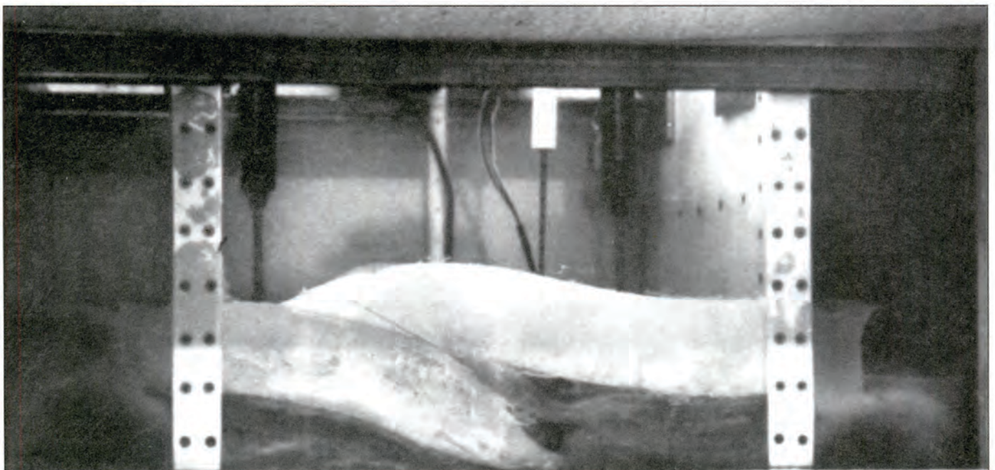
Figure 7. Photograph of final stage of described experiment. Two originally horizontal layers of paraffin wax were shortened by \sim 30\% . Width of photograph is 50 cm.
