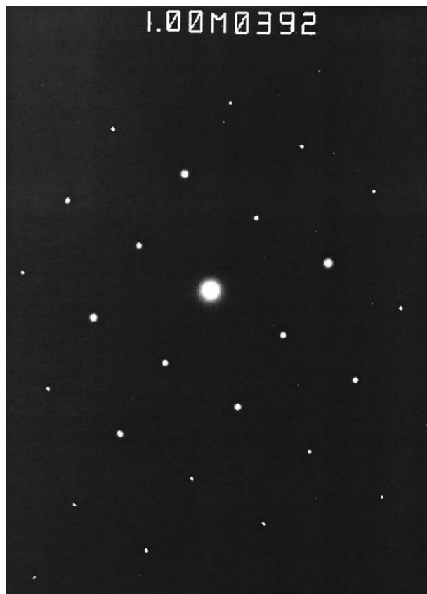
Fig. 4. Electron diffraction pattern obtained along [001] zone axis.
