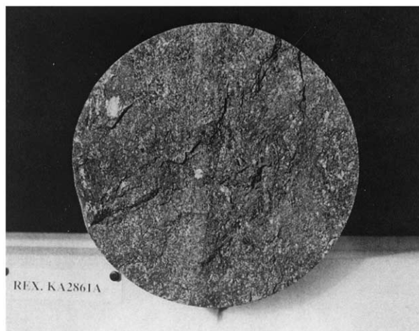
Fig. 1. Photograph of the fracture surface on the diorite core sampled in borehole KA2861A in the HRL at Äspö (diameter, 176 mm).
