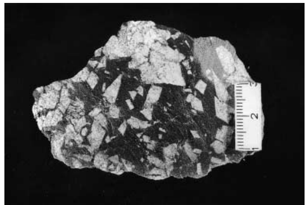
Fig. 3. Photograph of metarodinite with rhombic shaped, white pseudomorphs after lawsonite in a dark, chlorite rich matrix. Scale in cm.
