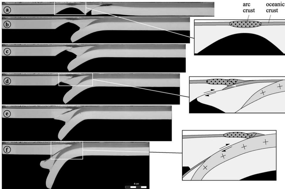
Fig. 4. Successive stages of experiment 1 with zoom-in of some parts of the deformed model. There is no young back-arc basin; therefore the overriding lithosphere contains only one thin zone beneath the arc. The lithosphere fails below the arc crust (panels b and c), resulting in the fore-arc block subduction (panels d–f). Only small parts of the fore-arc oceanic crust are scraped and accreted (zoom-ins in panels d and f). The arc crust is slightly deformed and remains in its place.
