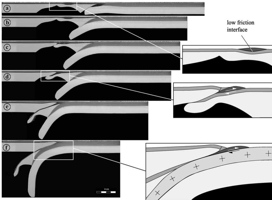
Fig. 7. Successive stages of experiment 4. The arc is strong, but there is a low-friction interface within it (zoom-in in panel a), which is a décollement surface along which the upper part of the crust is scraped off just at the onset of the arc subduction (panels d–f).
