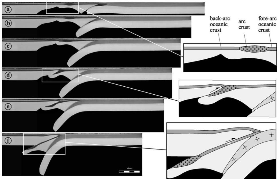
Fig. 5. Successive stages of experiment 2. The arc is thin and strong (corresponding to Fig. 3b). The arc subducts almost completely, leaving on the surface only small blocks of scraped off and accreted back-arc and arc crust (zoom-ins in panels d and f).
