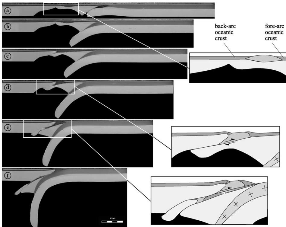
Fig. 6. Successive stages of experiment 3. The thin and weak ‘continental-like’ volcanic arc (corresponding to Fig. 3c) is deformed and accreted along with small amounts of the fore-arc oceanic crust (zoom-in in panel c).
