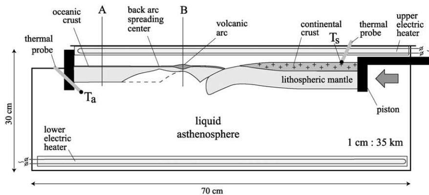
Fig. 2. Scheme of the experimental set-up. Dashed line in the lower part of the overriding plate shows the base of this plate in experiment 1 where young back-arc basin is absent.  $T_s$  and  $T_a$  are the temperatures of the lithosphere surface and the asthenosphere, respectively. Sections A and B correspond to the strength envelopes in Fig. 3.
