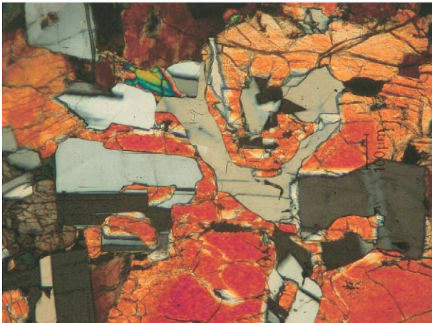
Fig. 4. Anorthite (white)-olivine (brown) intergrowth in transmitted light (A). Both phases are intimately intergrown, olivine is in places replaced by augite (dark brown). (B) Same as (A) but under crossed polarizers. Olivine has mostly the same optical orientation (consists of a single crystal) and anorthite forms many twinned individual grains.
