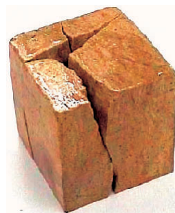
Fig. 7. Sample photo after fracture to show the fracture planes (sample: MD027).
