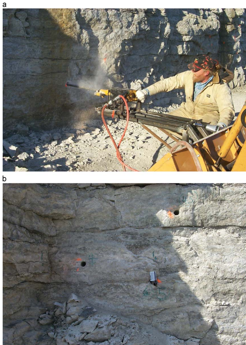
Fig. 2. (a) Horizontal drilling to insert conductive metal rods, 1.5 m in length and 4.4 cm in diameter; (b) a credit card serves as a scale for the horizontal holes.
