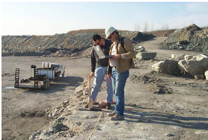
Fig. 4. GPR data were acquired on a flat limestone bench 1 m behind the quarry face with the 400-MHz antennas and 10-cm trace spacing.
