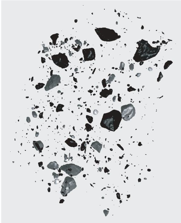
Fig. 2. Three-dimensional view of the crystals in sample F7-14B. Quartz crystals are shaded black; sanidine crystals are dark gray; magnetite is light gray. Glass and vesicles were suppressed for clarity. Field of view is \sim 8 \text{ mm} \times 7 \text{ mm} . An animated version of this figure is available at http://www.petrology.oxfordjournals.org .
