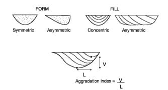
Fig. 2.—Terminology for describing the cross-sectional geometry of channel bodies. The origin of the terms is noted in Table 1.
