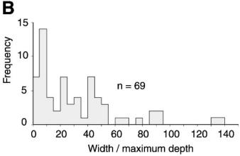
Fig. 14.— Width/depth measurements for modern channels. A) Width/mean depth for 278 surveyed reaches in Church and Rood (1983) and Hey and Thorne (1986), representing datasets from 16 publications; one value at 328 not shown. B) Width/maximum depth for 69 reaches in Schumm (1960). See Table 8 for information about these datasets.
