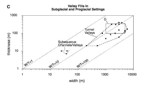
Fig. 9.—Width: thickness plots for valley fills. Studies used for the plots are listed in Appendix 1. Diagram format is explained in Figure 5. A) Valley fills on bedrock unconformities; O = Ocejo Formation (solid squares); M = Miocene-Pliocene of Italy and France; MG = Mannville Group; S = Sis Conglomerate; T = Miocene of Tuscany. B) Valley fills associated with alluvial and marine strata. C) Valley fills in subglacial and proglacial settings; D = tunnel valleys offshore Denmark.
