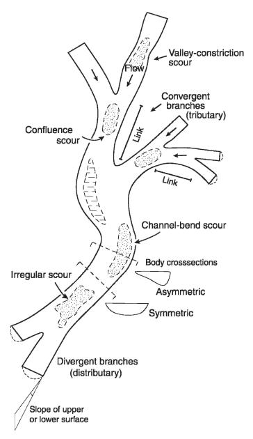
Fig. 3.— Terminology for describing the three-dimensional form of channel bodies. The diagram is based on valley fills with distinct branches and tributaries (e.g., Feldman et al. 1995; Plint 2002), but the terms may also be applicable to broad channel bodies with a complex history and internal geometry.
