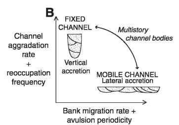
Fig. 15.—Conceptual diagram to show balance between factors that govern geometry of **A**) single-story channel bodies and **B**) multistory channel bodies.
