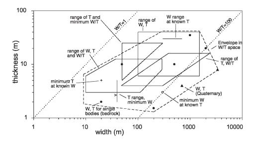
Fig. 5.—Construction methods for width: thickness plots. Note that general ranges of width and thickness reported by authors are represented by polygons, boxes, and triangles. However, width and thickness show a broad correlation, and upper left and lower right areas of these shapes are probably not occupied. Thus bounding envelopes for the datasets may cut through these areas if they project beyond other data points.
