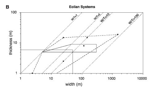
Fig. 8.—Width: thickness plots for A) Fixed river systems; Quaternary deposits from Rhine–Meuse system (open triangles) and Columbia River (solid triangles). B) Channels in eolian settings. Studies used for the plots are listed in Appendix 1. Diagram format is explained in Figure 5.
