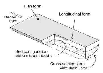
Fig. 1.— Geometric description of modern channel form. No scale implied. Modified from Knighton (1998).
