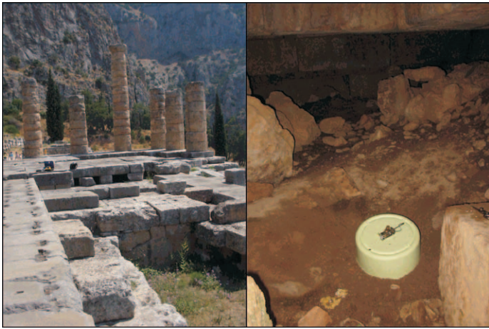
Figure 2. View of the Temple of Apollo and the site of the measurements in the Adyton (left); gas flux measurement by closed chamber on the soil inside the temple (right).
