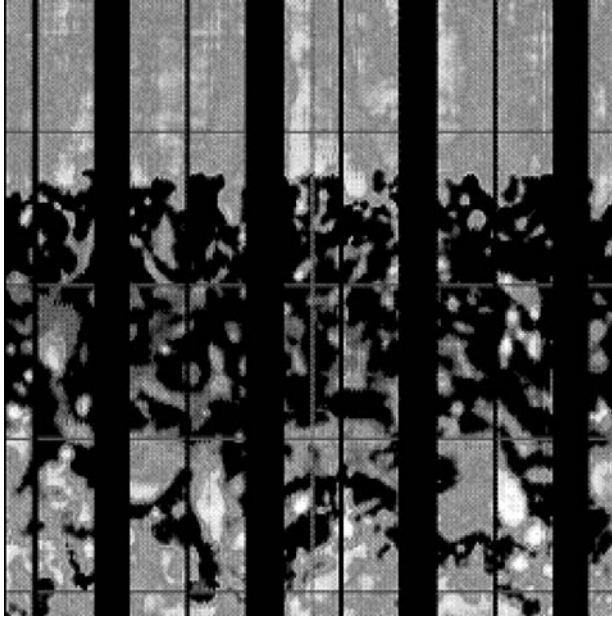
Figure 11. Porosity image of 24 in. high interval around the 26.7 in. circumference ( 8.5 \times \pi ) of the borehole. The horizontal grid lines have a vertical spacing of 6 in. Note the relatively large gaps between the four arms, and the relatively small gap between each pad-flap pair. The mean porosity of the interval is 22%. Black is relatively high porosity, while white indicates relatively low porosity. Note the very heterogeneous layer in the middle of the image comprising numerous 1–2 in. diameter vugs. Also note the abrupt contact above with a relatively homogeneous layer.
