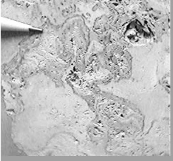
Figure 2. Photograph of hand sample of heterogeneous limestone. Some portions of the sample have very low porosity, while other portions are composed of empty vugs.
